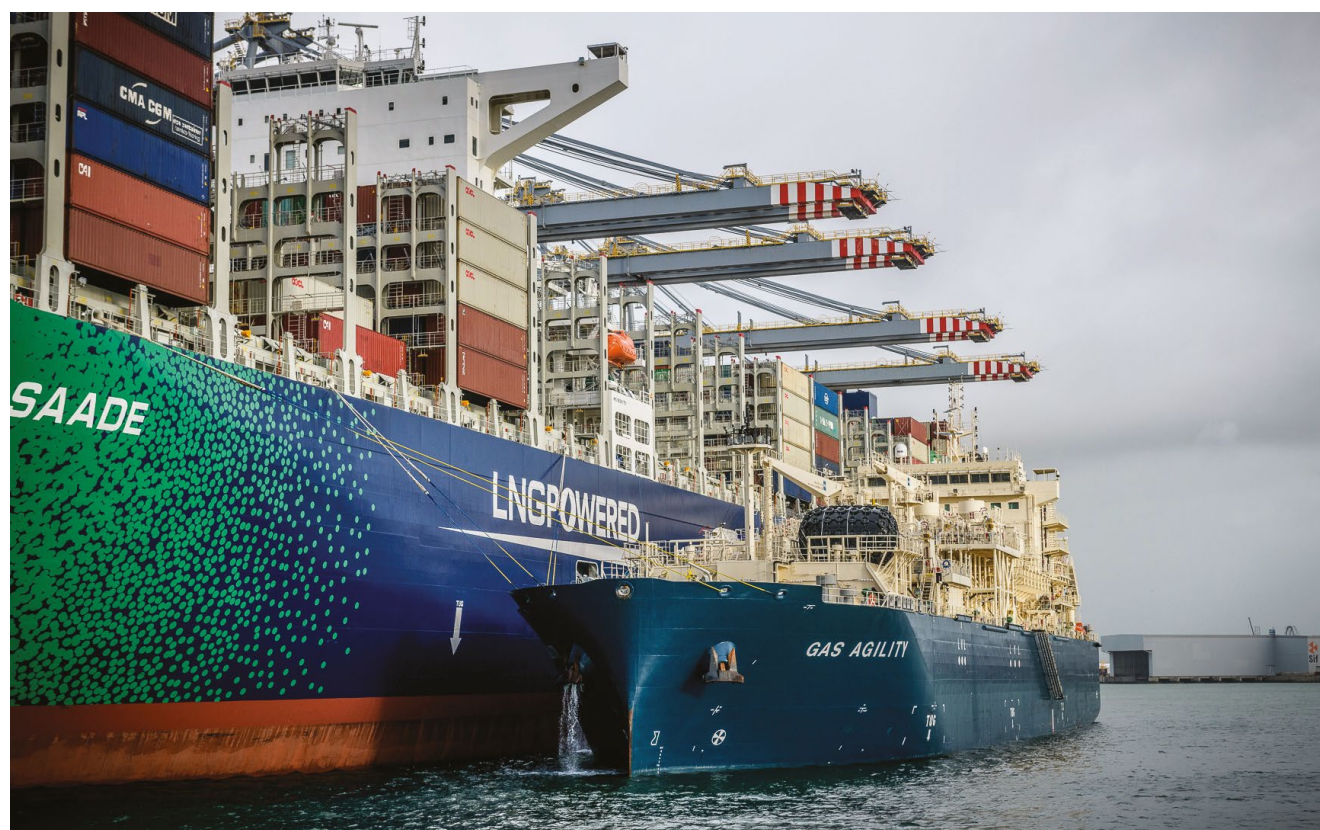
In November, Gas Agility, the largest bunker vessel in the world, performed the first bunkering in Port of Rotterdam for CMA CGM's Jacques Saade, the world's largest LNG-fuelled vessel, including 13% bio-LNG mix, supplied by SEA-LNG member Total.
