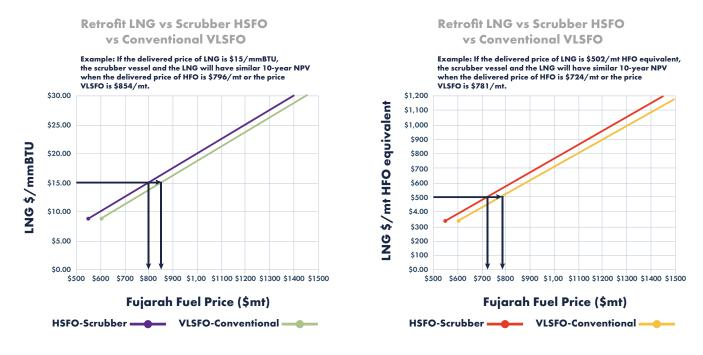
The charts above enable users to understand the relative fuel prices that will provide the same returns for different investment choices in the absence of a carbon levy. The left-hand chart shows LNG priced in energy units \$/mmBTU, and the right-hand chart provides LNG in \$/mt HFO equivalent based on lower heating value (LHV.)<sup>4</sup>
