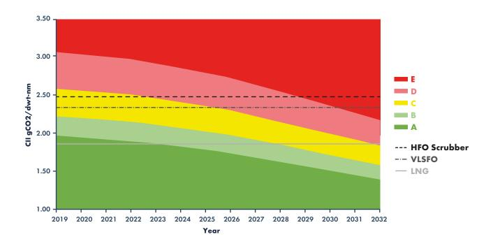
The chart displays the IMO CII grade ratings for VLCC retrofit alternatives: HFO scrubber, VLSFO and LNG fuel. HFO Scrubber falls from C to D year 2023 and into E mid-year 2028. Compliant VLSFO falls from C to D year 2025 and into E in the year 2030. LNG maintains superior rating B until it slides into C mid-2027 before finally slipping to D in 2032.
